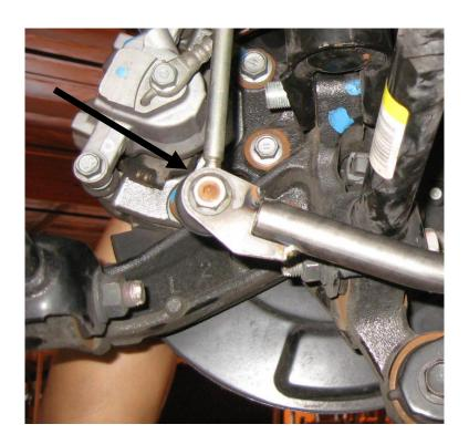
3. Locate the end link attached to the rear sway bar. Use a 6mmm allen wrench to hold the stud and box wrench to loosen the nut and separate the end link from the sway bar. Repeat on the opposite side.
