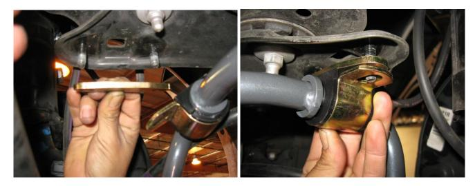
6. Place the backing plates under the new bushing and bracket as shown. Using the stock (OEM) hardware, attach the bar and brackets to the stock mounting locations. Torque the mounting hardware to 28 ft/lbs.
