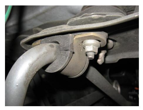
4. Next, locate the bushing brackets that attach the bar to the chassis. Remove the nuts that hold the bushing brackets and bar to the vehicle. Remove the bar and brackets, keeping the hardware.
