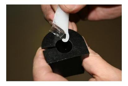
5. Locate the pivot "D shaped" polyurethane bushings and tube of special grease supplied in the hardware kit. Cut the end off of the grease tube and apply the grease to the bore of the polyurethane bushings (in the hole). Open the bushings and snap them over the new Progress Anti-sway Bar, as positioned on the stock bar.
